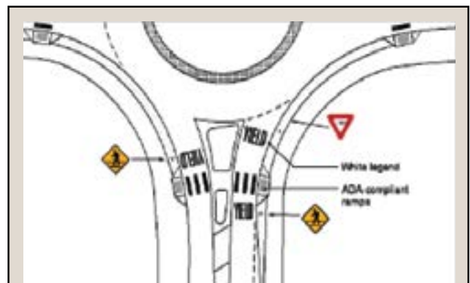
Figure E-11: Modern Roundabout Pedestrian Crosswalk Treatment
