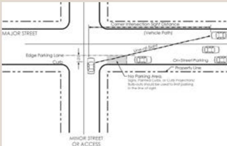
Figure 4-18: Corner Sight Distance (on-street parking)
