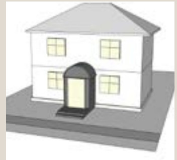
Portico with Arch Roof
