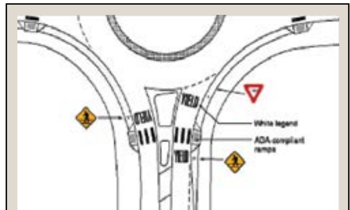
Figure E-11: Modern Roundabout Pedestrian Crosswalk Treatment
