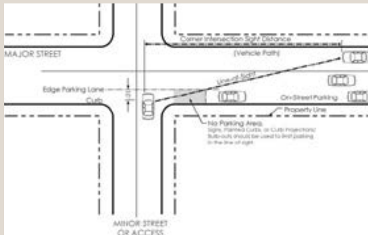
Figure 4-18: Corner Sight Distance (on-street parking)
