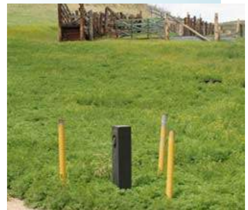
The Army Corps of Engineers has drilled monitoring wells in an effort to map the TCE groundwater plume at Belvoir.
