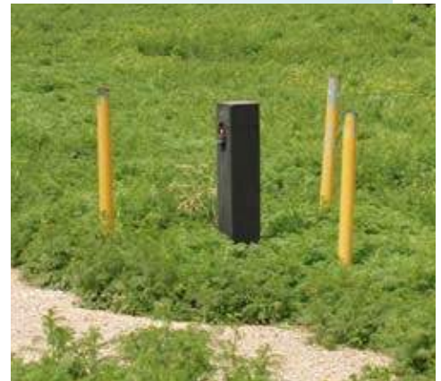
Monitoring wells are located throughout the Ranch, to help BOPU study how water development is affecting the aquifers.
