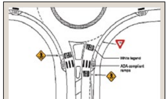
Figure E-11: Modern Roundabout Pedestrian Crosswalk Treatment
