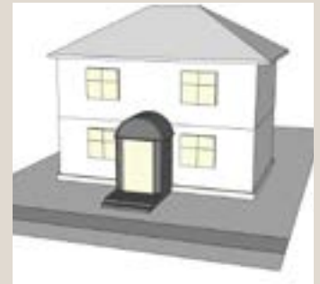
Portico with Arch Roof
